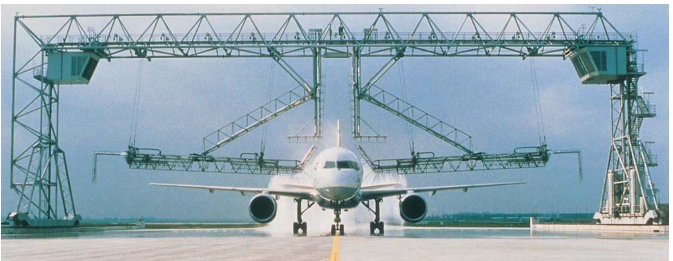
In this application Sigma Eurolock switches are combined with extra long flexible antennae to provide accurate position sensing for an airliner de-icing process. This is just one example from a vast number of diverse applications where the unique characteristics of Sigma switches mean they are the best (and sometimes only) choice.
